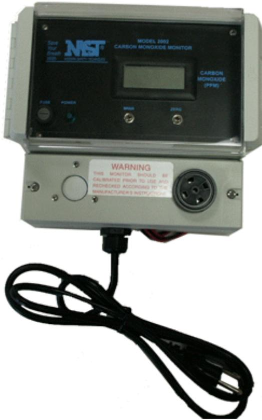
The *new* 2002 toxic gas monitor system is a cost effective, single point, fixed monitoring system for gas analysis. The monitor is housed in a NEMA 4 enclosure with clear front panel and digital readout, and is designed to operate in forced air, diffusion, or remote sensing modes - allowing the instrument to fit many applications for gas detection in non-flammable atmospheres.
